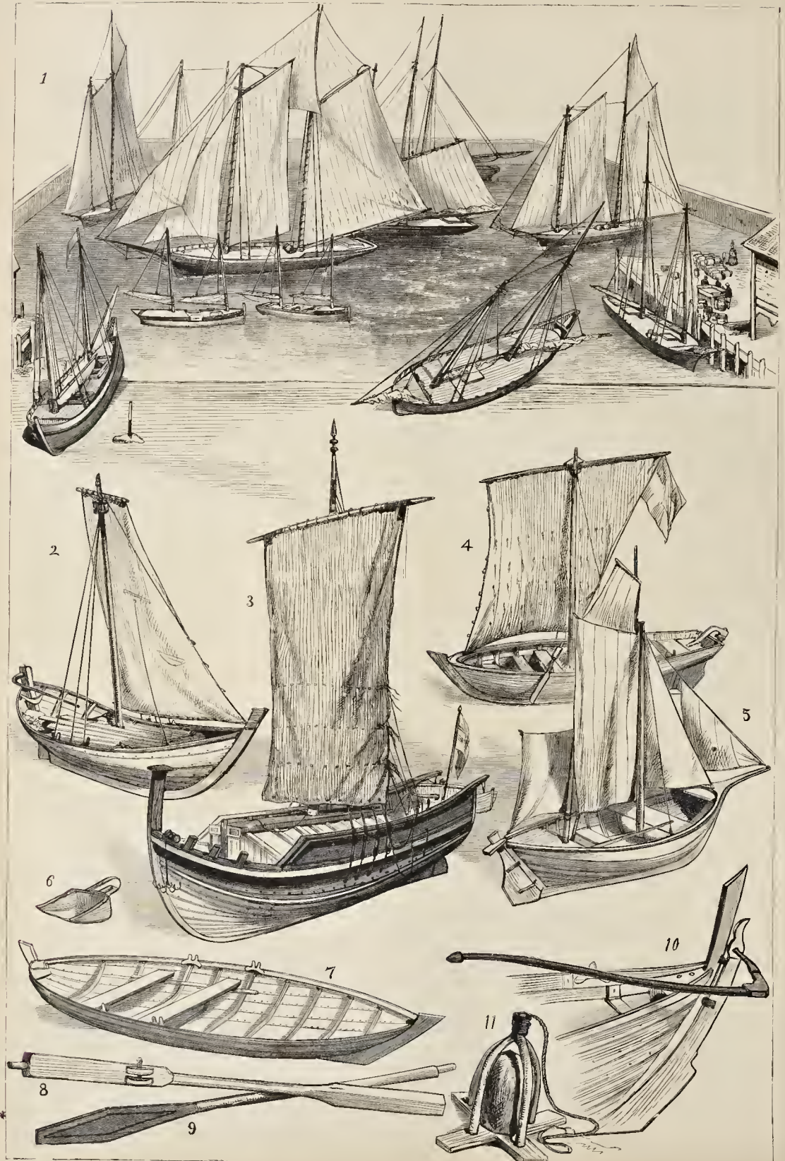
1. Gloucester Coddish boat 2. Norwegian Fishing-boats. 4, 5. Swedish Pohla-boats. 6. Swedish Scoop. 7. Swedish Row Boat. 8. Swedish Oar. 9. Norwegian Oar. 10. Norwegian Rudder. 11. Swedish Anchor.
